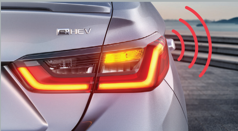
EMERGENCY STOP SIGNAL (ESS)
